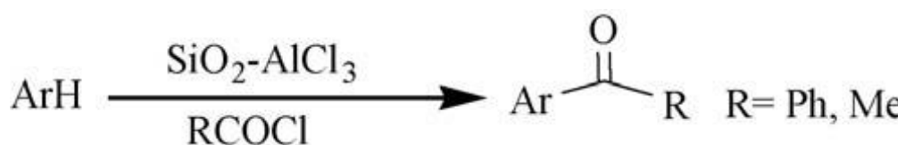
Scheme 1.5: Acylation of aromatic compounds with acid chlorides over SiO 2 /AlCl 3 .
