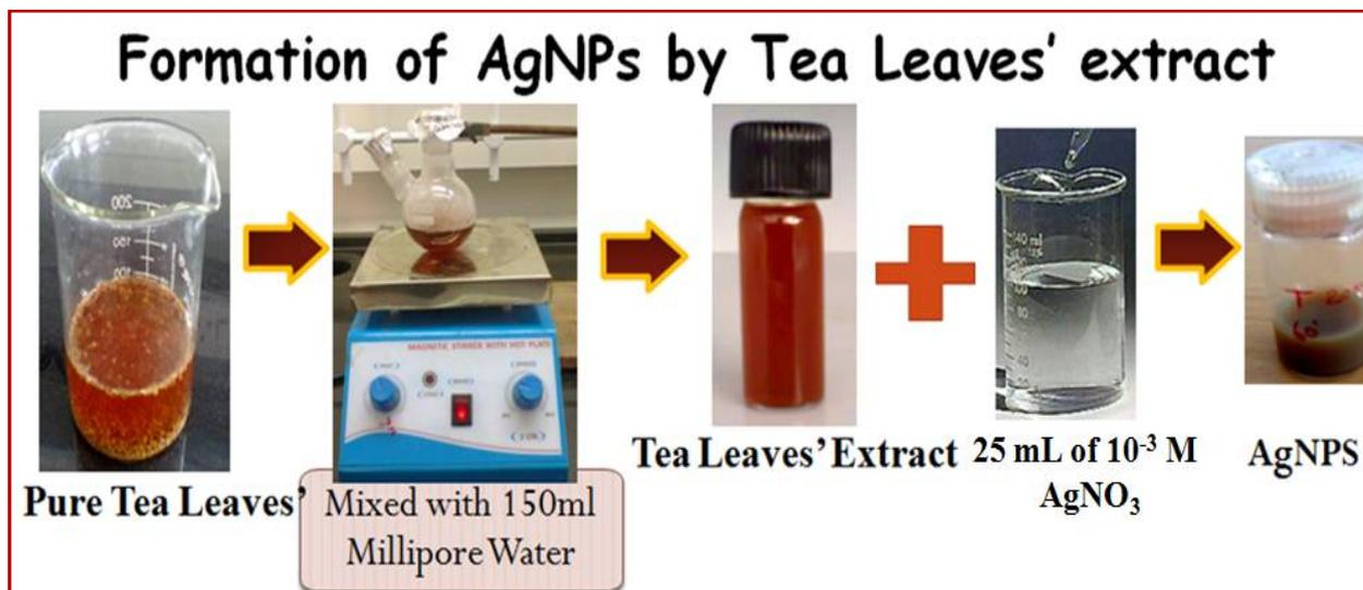
**Figure 3.19** Step-wise representation of the synthesis of AgNPs by Tea Leaves' Extract
