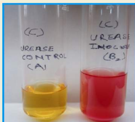
(F) Urease Production Test (25% FA Treated)
