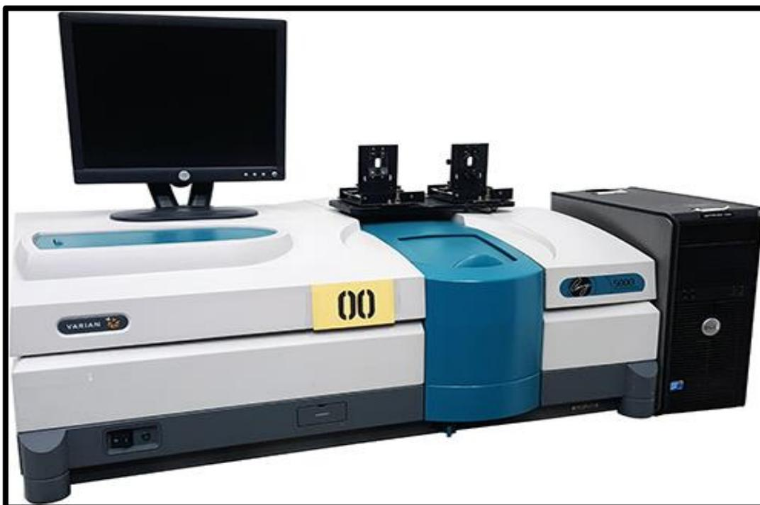
*Figure 2.8: UV-Vis Spectrophotometer*
