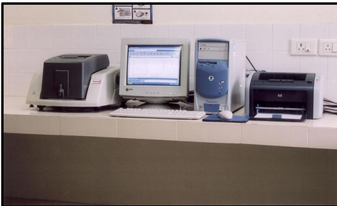
**Figure 2.7: FT-IR Spectrometer**
