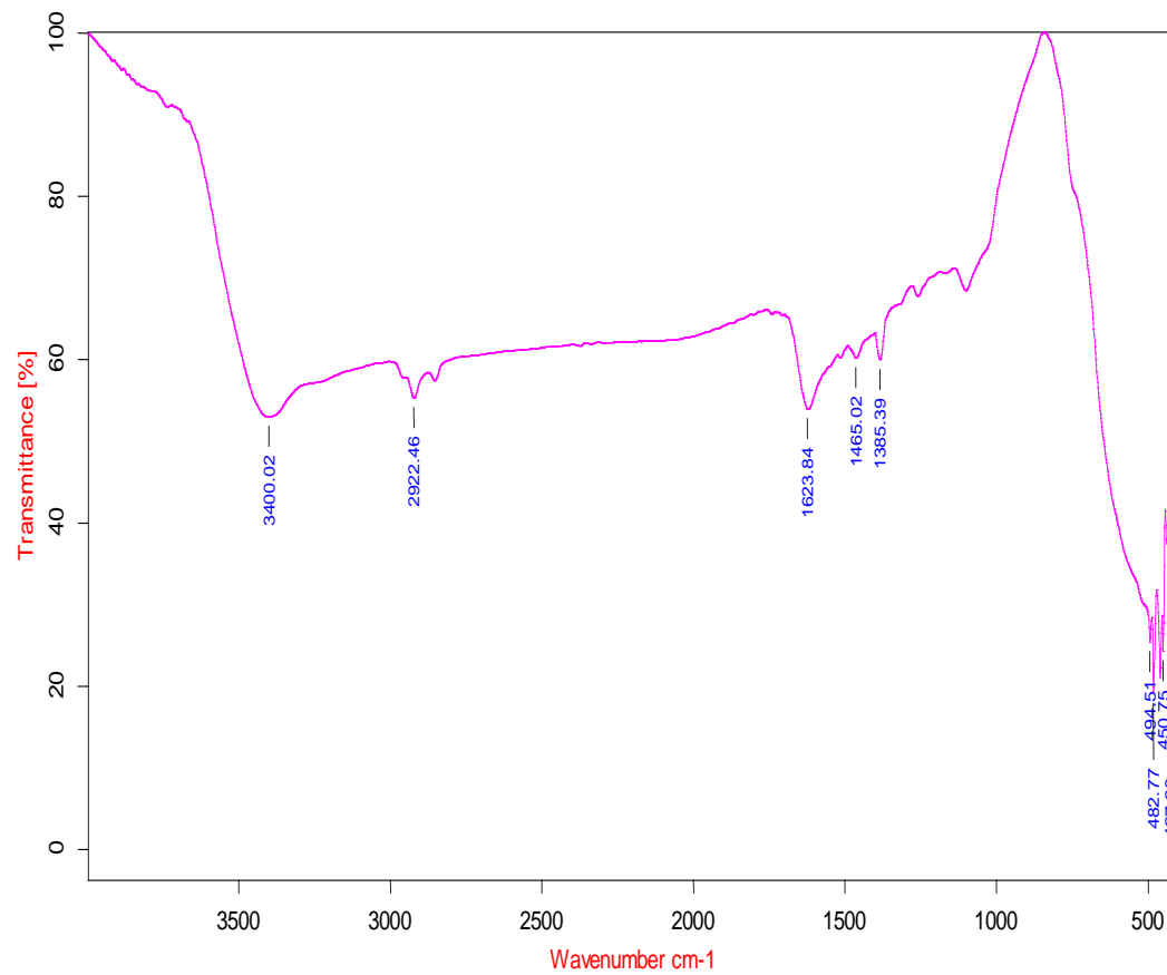
Figure 3.6: FT-IR spectra of synthesized colloidal MnO 2 .
