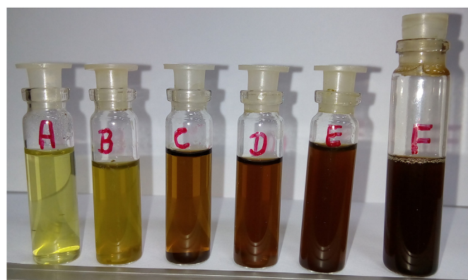
Fig. 1. Observation of color changes during synthesis of Copper nanoparticles at different time intervals: (A) 0 h, (B) 4 h, (C) 10 h, (D) 18 h, (E) 24 h, (F) 28 h. (For interpretation of the references to color in this figure legend, the reader is referred to the Web version of this article.)
