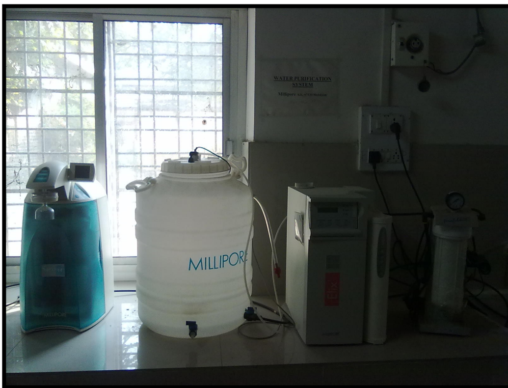
Figure 17: Ultra Pure Water Purification System (Elix UV3)
