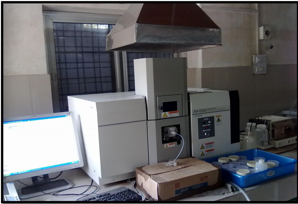
Figure 16: Atomic Absorption Spectrophotometer – Shimadzu-6300
